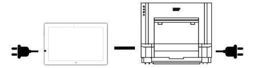
Make sure all power supply cables (Printer and Tablet) are connected. Now, please connect the tablet to the printer with the USB cable provided in the printer box.
